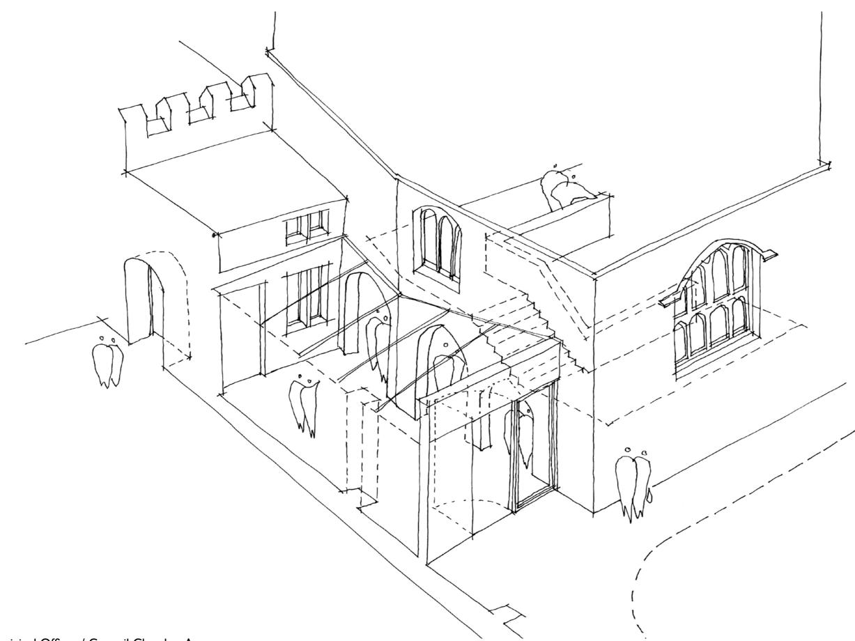
Municipal Offices / Council Chamber Access Proposed new glazed entrance to the Municipal Offices. A separate entrance has been maintained and provided through the existing single storey Porter's office. This involves removing a section of wall to the front which faces the existing route alongside the Guildhall and removing the roof. It will be replaced with a set back glazed link held off the junction with the Guildhall.
