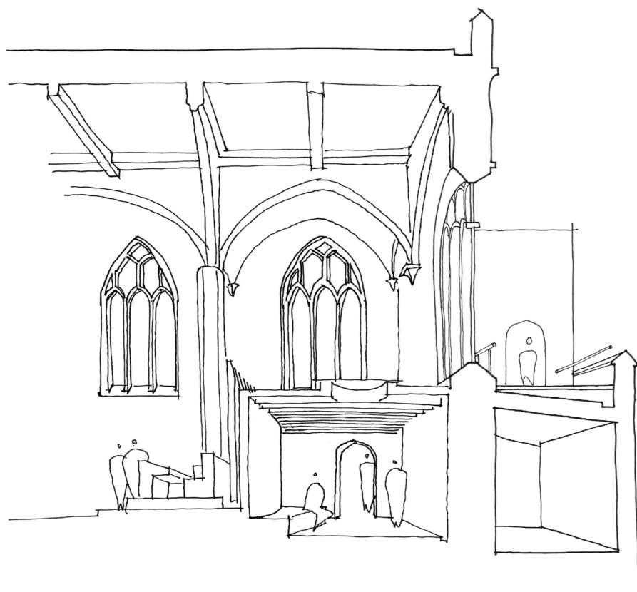
The Guildhall: screened passage and ramped access The new ramp to the southern end of the Guildhall resolves the problems with the circulation and levels to Committee Room 1, the South Range and the Municipal Offices. The ramp sits within an acoustic enclosure separated from the main Guildhall by a curving screen of oak, which acts as a new back drop to the relocated dais.
